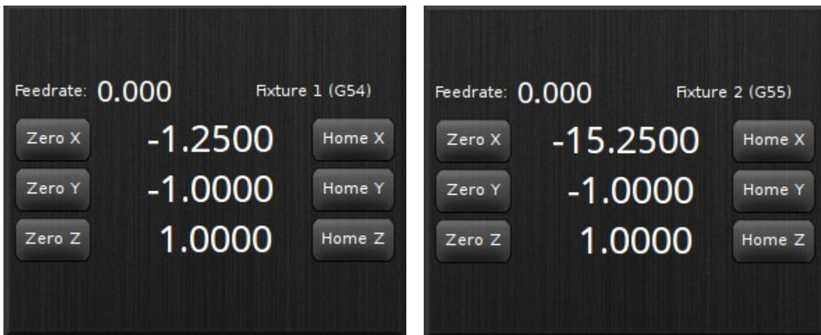
In the images above the tool is actually in the machine home position, which is machine zero (0, 0). When Fixture 1 is selected, the position in the DROs now shows (-1.25, -1.0), and when Fixture 2 is selected the position in the DROs changes to (-15.25, -1.0) – even though the machine has not moved.
